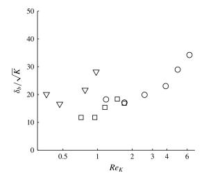
FIGURE 8. The  $Re_K$  dependence of the Brinkman layer thickness  $\delta_b$  normalised by  $\sqrt{K}$ : d=6 mm ( $\nabla$ ); d=10 mm ( $\square$ ); d=25 mm ( $\bigcirc$ ). The generally accepted proportionality of  $\delta_b \propto \sqrt{K}$  is not fully observed here, with  $\delta_b/\sqrt{K}$  increasing with  $Re_K$ .
