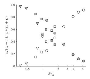
FIGURE 11. Partitioning of the fluid shear stress at the SWI as a function of  $Re_K$ : d = 6 mm ( $\nabla$ ); d = 10 mm ( $\square$ ); d = 25 mm ( $\bigcirc$ ). The individual stress components, viscous stress  $\tau_v$  (grey) and turbulent stress  $\tau_t$  (white), are normalised by their sum. The turbulent stress is negligible at low  $Re_K$ , but exceeds the viscous stress above  $Re_K \simeq 1-2$ .
