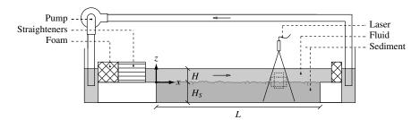
FIGURE 3. Experimental set-up of the recirculating flume. The flow is driven by a centrifugal pump and has a fixed depth of H=9 cm. The model sediment bed, consisting of monodisperse borosilicate glass beads, has a height  $H_s=15$  cm and a length L=1.1 m.
