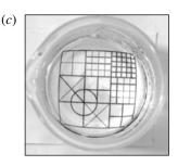
FIGURE 4. The refractive index matching combination of fluid and model sediment used in this study. Shown are borosilicate glass beads in (a) water, (b) 50% NaI solution, (c) 59% NaI solution. As the refractive index of the glass beads and the fluid are equal in (c), the image underneath the fluid remains undistorted. The 59% NaI solution was used in experiments.
