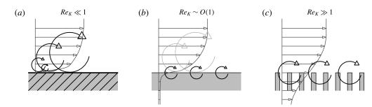
FIGURE 2. Framework identifying flow at the SWI (b) as a transition between flows over impermeable boundaries (a) and highly permeable boundaries (c). The variation of the structure of the mean flow and turbulence with  $Re_K$  is shown schematically.
