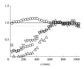
FIGURE 5. Flow statistics along a longitudinal transect 20 mm above the SWI:  $\langle \overline{u} \rangle$  ( $\bigcirc$ ),  $\sigma_u$  ( $\square$ ),  $\sigma_w$  ( $\nabla$ ),  $\langle \overline{u'w'} \rangle$  ( $\triangle$ ). The statistics are normalised by the average value in the range 700 < x < 800 mm, where x = 0 corresponds to the leading edge of the sediment bed. Fully developed flow at the interface is reached by x = 600 mm.
