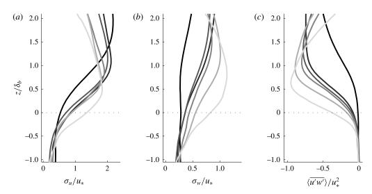
FIGURE 9. Turbulence statistics for six cases (S2, S3, M7, L11, L12, L14; from black to grey respectively) with varying  $Re_K$ : (a) streamwise turbulence intensity, (b) vertical turbulence intensity, (c) Reynolds stress. Vertical distance is normalised by the Brinkman layer thickness ( $\delta_b$ ) and turbulent velocities by the shear velocity ( $u_*$ ). The normalised turbulence intensities and the turbulent shear stress at the SWI increase monotonically with  $Re_K$ .
