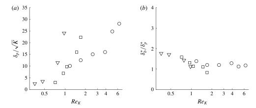
FIGURE 12. (a) The increase of the normalised shear penetration depth  $(\delta_p/\sqrt{K})$  with  $Re_K$ : d = 6 mm ( $\nabla$ ); d = 10 mm ( $\square$ ); d = 25 mm ( $\bigcirc$ ). (b) Comparison of the shear stress penetration depth to the flow penetration depth, both relative to  $z_U$ , suggesting transitional behaviour above  $Re_K \simeq 1-2$   $(\delta_h^*/\delta_n^* \simeq 1.25)$ .
