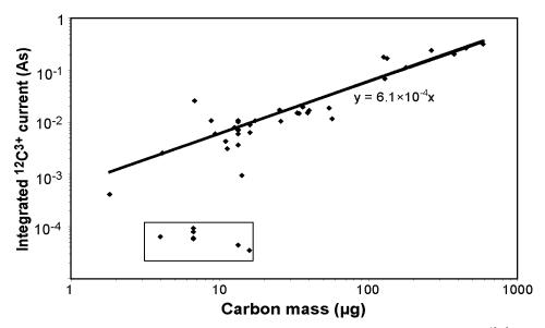
Figure 5 Indication of the analytical sensitivity of graphitization and AMS measurement. The integrated  ${}^{12}C^{3+}$  current is shown for all completely sputtered samples versus the carbon mass calculated from the CO<sub>2</sub> pressure before graphitization. The slope of the linear fit corresponds to a total detection efficiency of 2.1%. The deviating data points in the box are discussed in the text.
