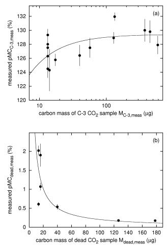
Figure 4 Contamination during  $CO_2$  graphitization and AMS measurements. Measured pMC values for a) IAEA C-3  $CO_2$  and b) dead  $CO_2$  are plotted versus carbon mass of processed  $CO_2$ . Note that contamination with unknown pMC leads for small standard amounts to measured pMC values that are too low (a). For small blanks, the measured pMC values are too high (b). The curves shown are model fits that allow one to assess the carbon contamination.
