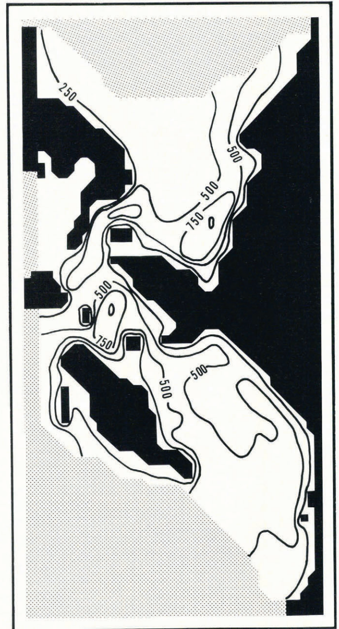
Fig. 2. Initial configuration of the grid used in the West Antarctic study. The shaded pattern represents open water, the black region represents grounded ice, and the white area represents floating ice. The contours represent sea-bed depths in meters below sea-level, as they would exist if the present West Antarctic ice cover were removed and isostatic rebound occurred. These are smoothed from sheet 6 of Drewry (1983).
