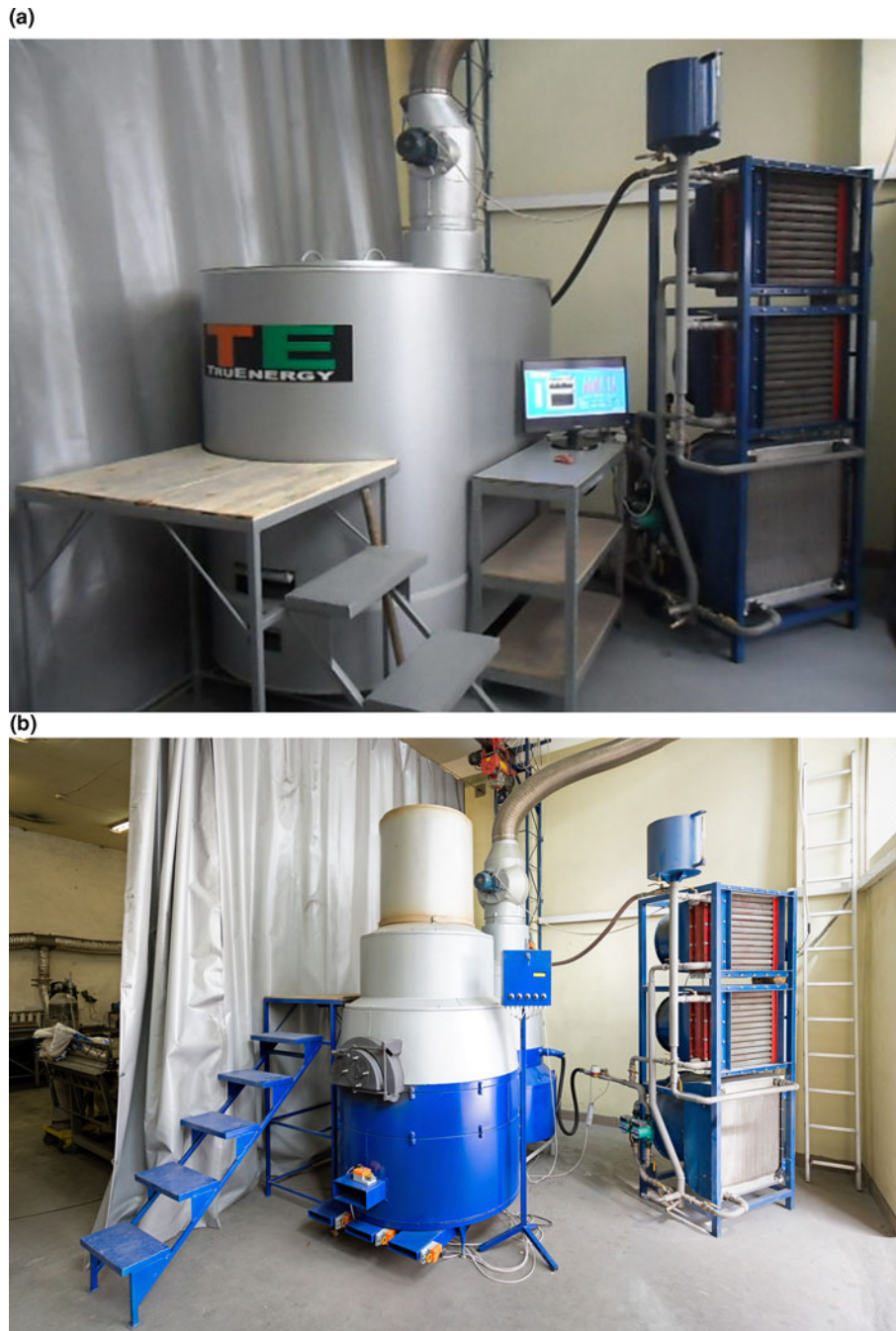
Figure 1. Our gasifiers of 2016 (a, which recycles 30 kg/h of waste) and of 2018 (b, which recycles 80 kg/h of waste).
