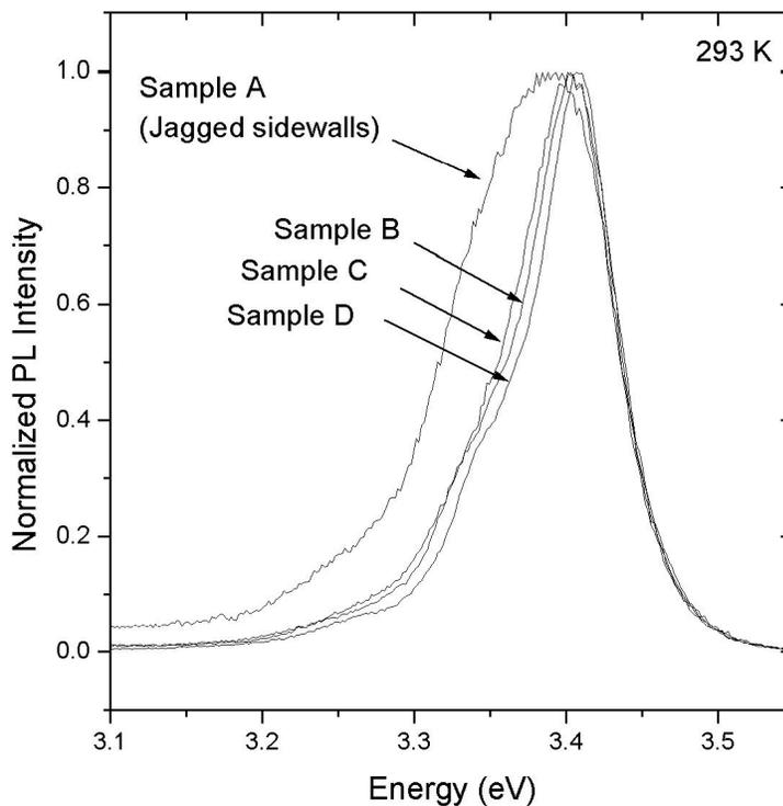
Figure 4 Room-temperature PL of samples A-D.
