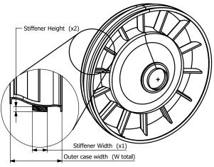
Figure 2. Schematic of the TRS and deposited stiffener
