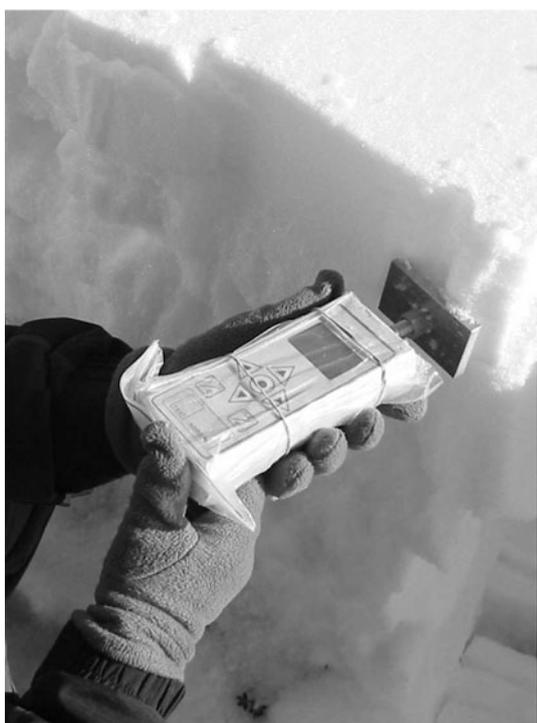
**Fig. 2.** Push-pull gauge with connected fist attachment.
