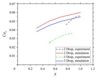
Figure 16. Phase boundary plots as obtained from BEM and experiments for both two and three droplet systems.
