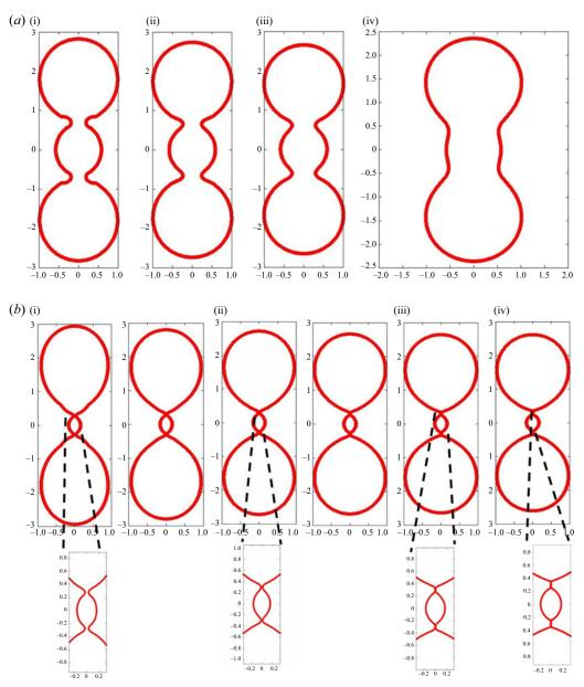
Figure 15. (a) Coalescence after bridging three droplet system obtained for Ca = 0.15, for  $R_2/R_3 = 0.6$ , for non-dimensional times (i) t = 0, (ii) t = 0.005, (iii) t = 0.01, (iv) t = 0.02. (b) Non-coalescence after bridging three droplet system obtained for Ca = 0.15, for  $R_2/R_3 = 0.2$ , for non-dimensional times (i) t = 0, (ii) t = 0.005, (iii) t = 0.005, (iii) t = 0.01, (iv) t = 0.02.
