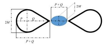
Figure 5. Estimation of symmetric and asymmetric deformation.
