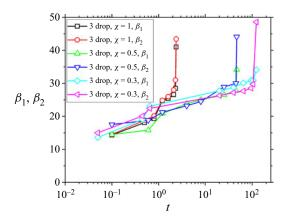
Figure 11. Numerically obtained variation of cone angles at contact with non-dimensional time (*t*) for three droplet system under an electric field where  $\beta_1$  and  $\beta_2$  are the angles subtended by droplet 1 and droplet 2, respectively.
