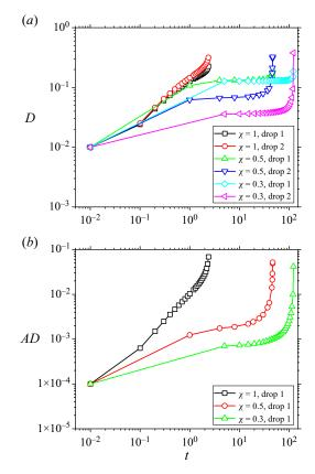
Figure 10. (a) Numerically obtained variation of symmetric deformation (D) of individual droplets under electric field with non-dimensional time (t) in a three droplet system. (b) Numerically obtained variation of asymmetric deformation (AD) of individual droplets under electric field with non-dimensional time (t) in a three droplet system.
