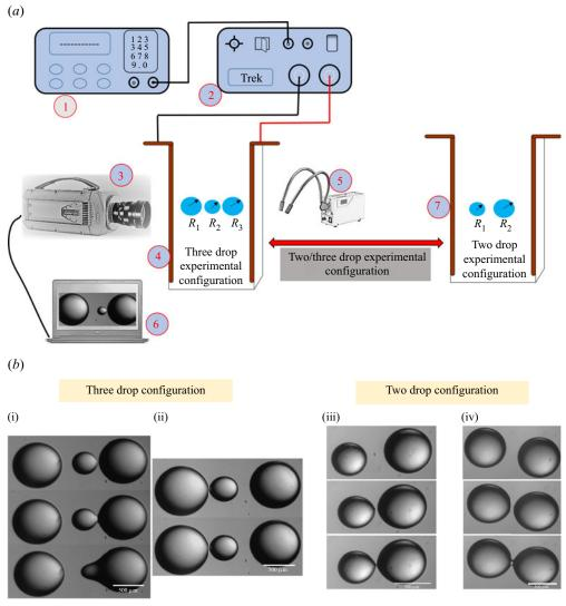
Figure 1. (a) Experimental set-up to study interactions of two or three aqueous droplets suspended in silicone oil. (b) (i) Three aqueous droplets undergoing coalescence: Ca = 0.024, (ii) three aqueous droplets undergoing non-coalescence: Ca = 0.04 (iii) two aqueous droplets undergoing non-coalescence: Ca = 0.043 and (iv) two aqueous droplets undergoing coalescence: Ca = 0.044. Scale bar is 500 µm. Here, the radius ratio is  $\chi = R_2/R_1$ .
