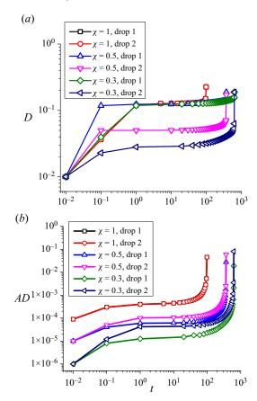
Figure 7. (a) Numerically obtained variation of symmetric deformation, (D) of individual droplets under electric field with non-dimensional time (t) in two droplet system. (b) Numerically obtained variation of asymmetric deformation, (AD) of individual droplets under electric field with non-dimensional time in two droplet system.
