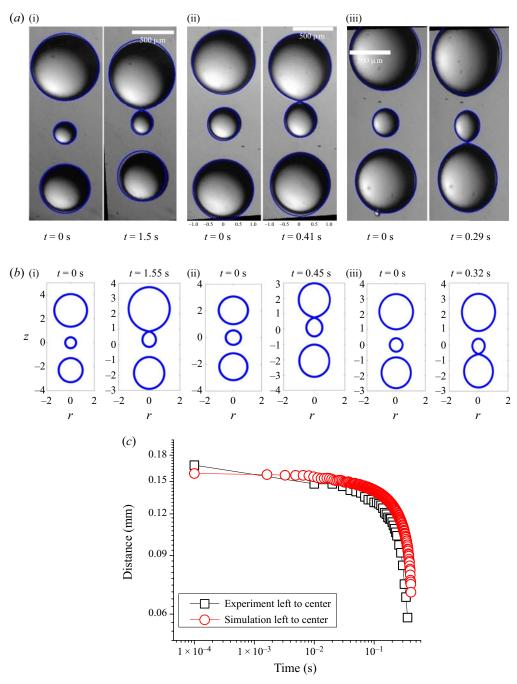
Figure 4. (a) Experimental (BEM superimposed) and (b) BEM prediction for DI water droplet in silicone oil at time t = 0 and at time t =contact, for (i) Ca = 0.033, (ii) Ca = 0.036 and (iii) Ca = 0.038. (c) Numerically and experimentally obtained variation of separation distance with time for a three droplet system under an electric field with Ca = 0.036 and  $R_2/R_1 = 0.51$ .
