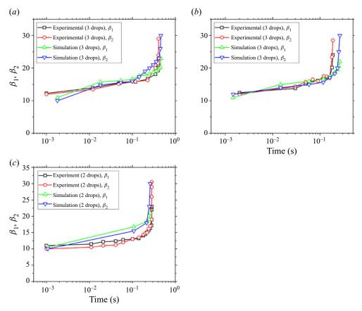
Figure 12. Comparison of variation of numerically and experimentally obtained cone angles at the peak of AC voltage under electric field with time for three droplet and two droplet systems. (*a*) Three droplet system: Ca = 0.036,  $R_2/R_1 = 0.51$ . (*b*) Three droplet system: Ca = 0.035,  $R_2/R_1 = 0.43$ . (*c*) Two droplet system: Ca = 0.063,  $R_2/R_1 = 0.7$ .
