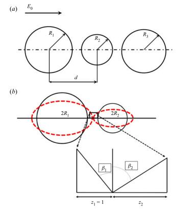
Figure 2. Schematic for (*a*) droplets under electric field and (*b*) the Bird *et al.* (2009) model modified to analytically solve for asymmetric cone formation with two cone angles  $\beta_1$  and  $\beta_2$ .
