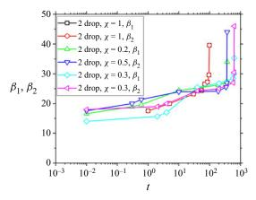
Figure 8. Numerically obtained variation of cone angles at contact with non-dimensional time (*t*) for two droplet system under electric field where  $\beta_1$  and  $\beta_2$  are the angles subtended by droplet 1 and droplet 2, respectively.
