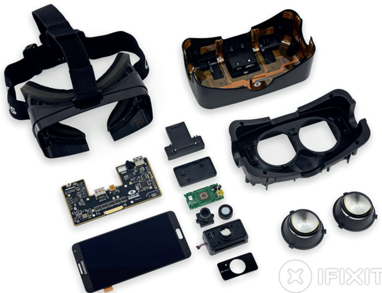
Figure 2.12 Disassembly of the Oculus Rift DK2 headset
