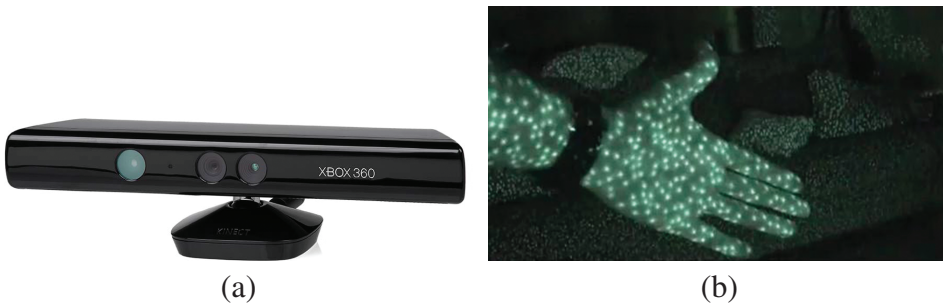
Figure 2.10 (a) The Microsoft Kinect sensor gathers both an ordinary RGB image and a depth map (the distance away from the sensor for each pixel). (b) The depth is determined by observing the locations of projected IR dots in an image obtained from an IR camera.
