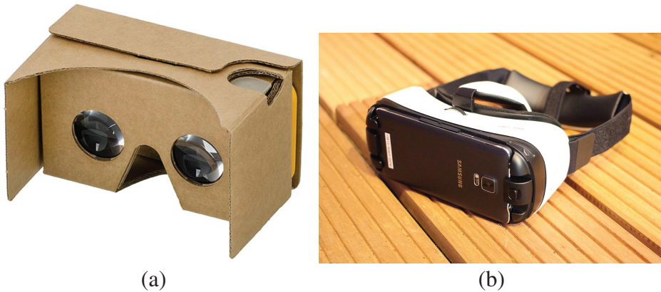
Figure 2.11 Two headsets that create a VR experience by dropping a smartphone into a case. (a) Google Cardboard works with a wide variety of smartphones. (b) Samsung Gear VR is optimized for one particular smartphone (in this case, the Samsung S6).
