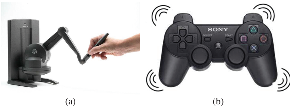
Figure 2.8 Two examples of haptic feedback devices. (a) The Touch X system by 3D Systems allows the user to feel strong resistance when poking into a virtual object with a real stylus. A robot arm provides the appropriate forces. (b) Some game controllers occasionally vibrate.
