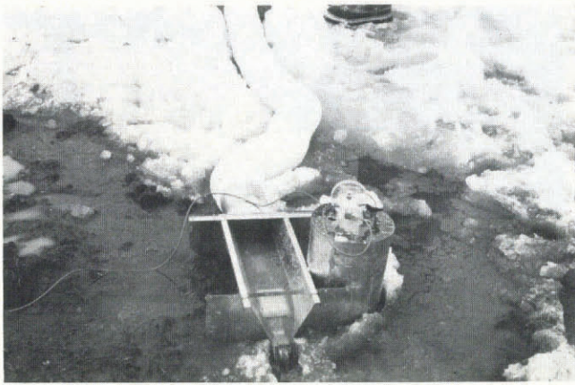
Fig. 6. Photograph of the flume and stilling well in operation.
