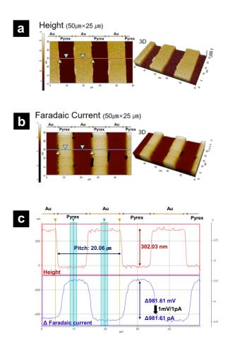
**Figure 1.** Representative SICM-SECM images. a) SICM topography image; b) SECM Faradaic current image. c) Line profile along the line seen in a) and b). Image size:  $50 \mu m \times 25 \mu m$ .
