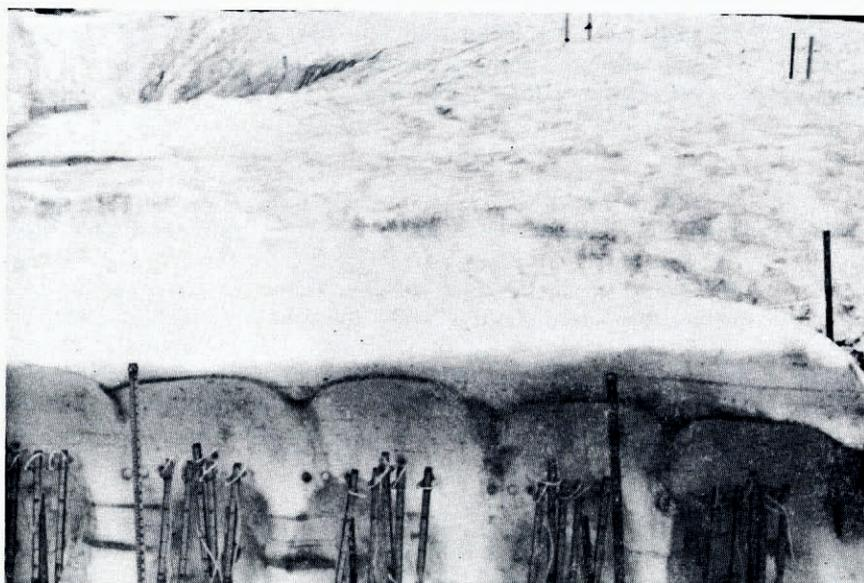
Fig. 2. A row of tensiometers installed in a melting snow-pack. One tensiometer in each group of five is installed about 50 mm higher than the others so that vertical pressure gradients can be measured. A metre stick is on the lower right (12 July 1974).
