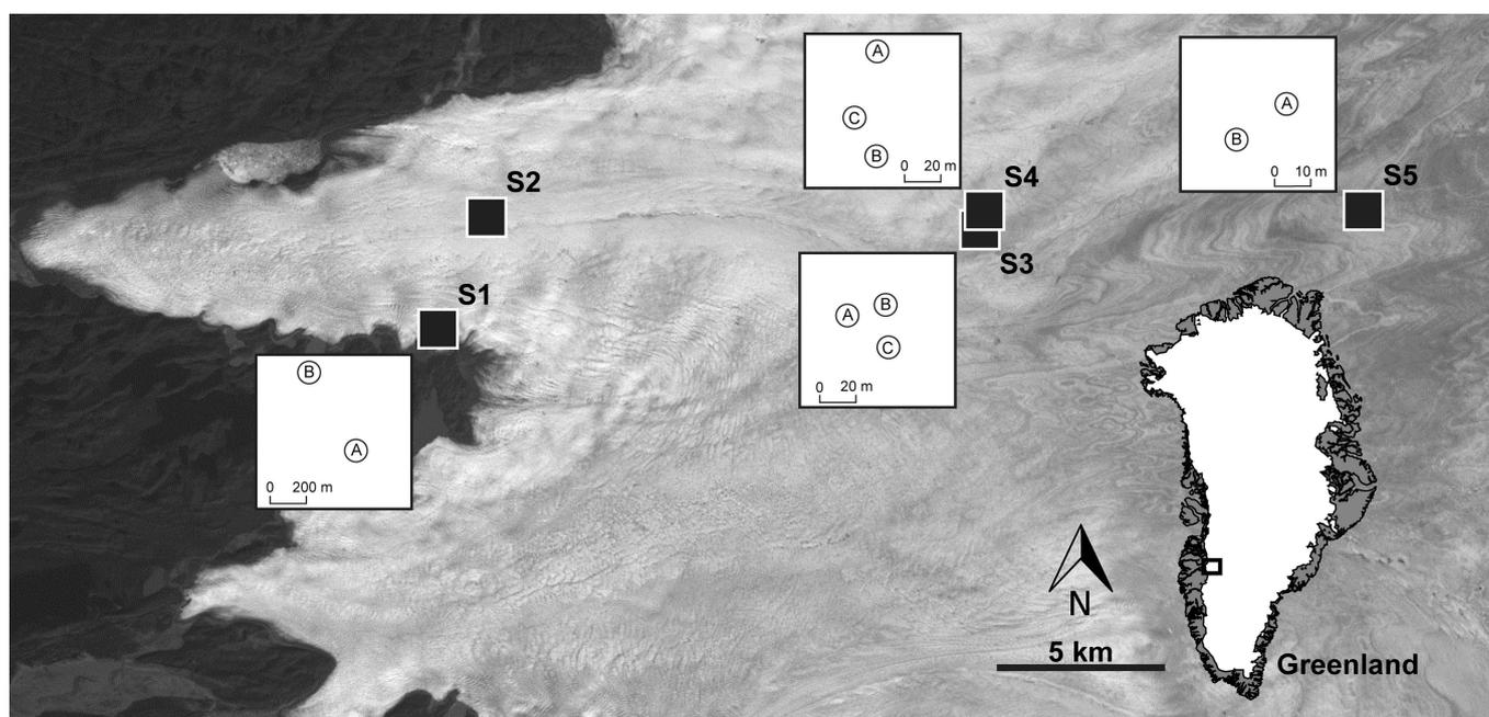
**Fig. 1.** Location of five drilling sites. Inset boxes show spacing of temperature profiles at each site. Flow directions for this region available in Jezek and others (2013).
