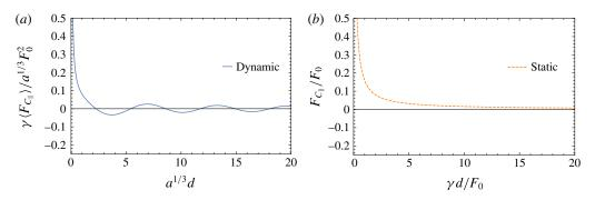
FIGURE 4. (Colour online) Lateral capillary force  $\langle F_{C_{\parallel}} \rangle$ , averaged over one period, between two dynamic (*a*) and static (*b*) point forces acting in the direction normal to a planar free surface, as a function of their separation distance *d*. In the dynamic case, the lateral capillary interaction has multiple equilibrium points, both stable and unstable, as the sign of the force oscillates between attractive and repulsive.
