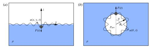
FIGURE 1. (Colour online) Schematic picture of the problems considered in the present paper: (a) dynamic point force acting on a planar gas-liquid interface, (b) dynamic point force acting on a bubble. The deformation of the free surface (dashed line) and the size of the particle are exaggerated for clarity.
