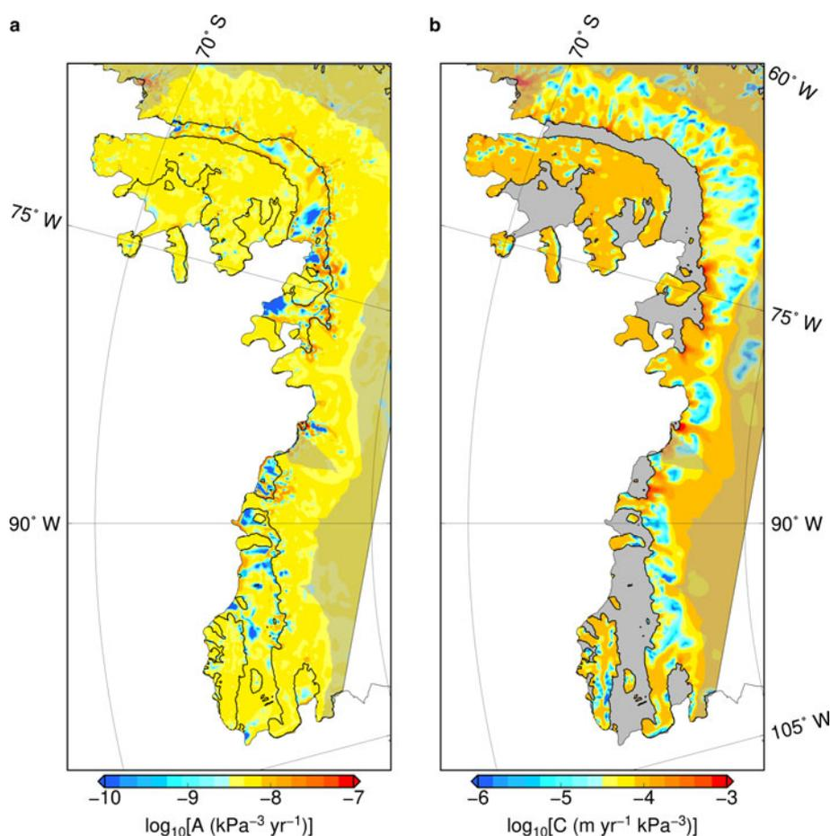
**Fig. 4.** Inferred ice rheology and basal slipperiness fields. (a) Rate factor  $A$  from the flow law (Eqn 1). (b) Basal slipperiness defined from the basal boundary condition (Eqn 2). Values of  $C$  over the ice shelves are irrelevant, and therefore shown in gray, because we impose  $|\tau_b| = 0$  where ice is afloat. Gray shaded regions are the same as in Figure 1b.
