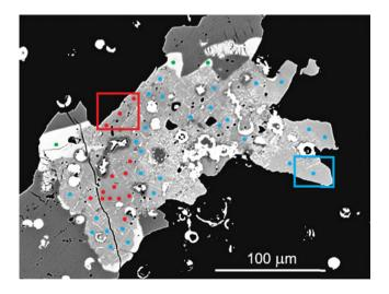
**Figure 1.** Back-scattered electron (BSE) image of the sample studied containing arsenoústalečite (red circles), stibioústalečite (blue circles), hakite-(Hg) (green circles), berzelianite (dark grey in BSE) and uraninite (white in BSE). The grains used for single-crystal X-ray diffraction study were extracted from the red (arsenoústalečite) and blue (stibioústalečite) boxes. Holotype sample.
