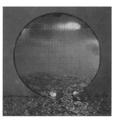
**ON THE COVER:** A 200 mm (8 inch) diameter silicon wafer with copper interconnections. The copper interconnection structure was developed and fabricated by members of IBM's Research Division and Microelectronics Division. The photograph was taken by D.C. Edelstein and E.G. Colgan. For more information about this topic, see "Materials Issues in Copper Interconnections" by J.M.E. Harper and colleagues on p. 23.
