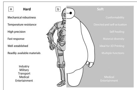
**Figure 2.** Selected properties and applications of traditional hard robots versus soft robots. The cartoons represent (a) a famous metallic humanoid<sup>4</sup> and (b) a soft character.<sup>11</sup>
