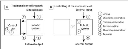
Figure 5. Controlling paths in robotic systems: (a) in traditional paths and (b) in future stiff composite robots, where the controls are decentralized at the materials' level. The blank square in (b) indicates the absence of an external control unit.
