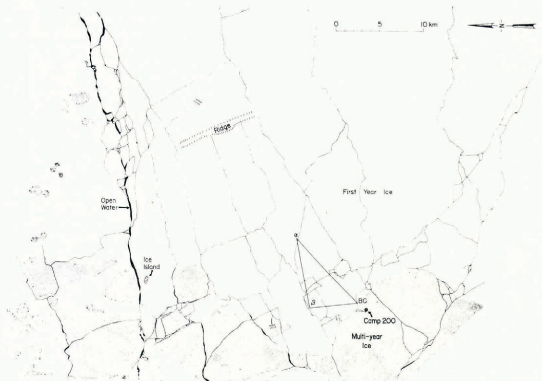
Fig. 2. Overlay of a photo mosaic showing the location of the strain array relative to the major fractures in the area near Camp 200 on 15 March 1971. This photography was obtained by NASA at an altitude of 10 600 m. Multiyear ice, annual ice, and ice islands were identified by variations in surface roughness.
