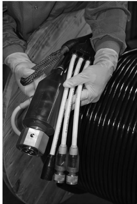
Fig. 7. Detail of the return water pump and instrumentation cable termination.
