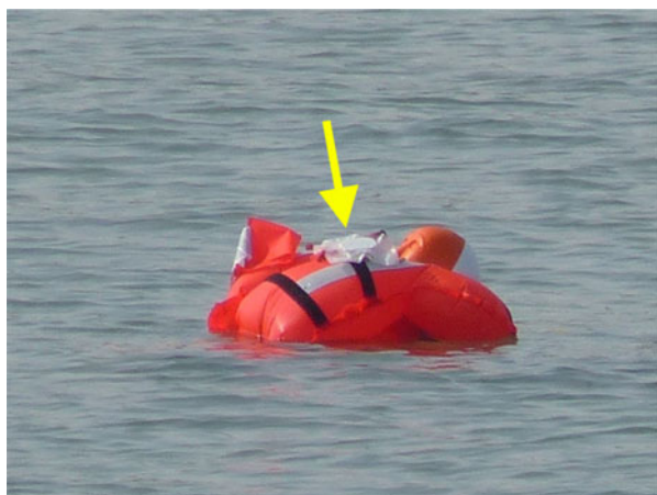
Fig. 29. Picture of the weighted body simulator wearing the inflatable life jacket floating in the water. Tag position highlighted, distance of the tags to the waterline approximately 20 cm.
