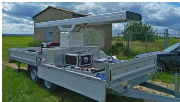
Fig. 23. Picture of the harmonic radar interrogator system including the S-/C-band antenna and the gearbox assembly mounted to a trailer during the final system trials on land at the Fraunhofer FHR in Wachtberg.
