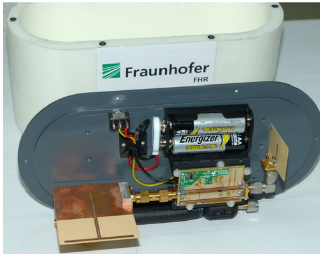
Fig. 12. Picture of the first active stand-alone BJT S-band to C-band frequency doubler tag prototype, without the integrated antennas or an additional LNA. Planar microstrip fed S-/C-band half-wave dipole antennas, ROHACELL radome, and mounting back-plate made by the Fraunhofer FHR. G_{RX} = 5 dBi H-polarized, G_{TX} = 4 dBi V-polarized.
