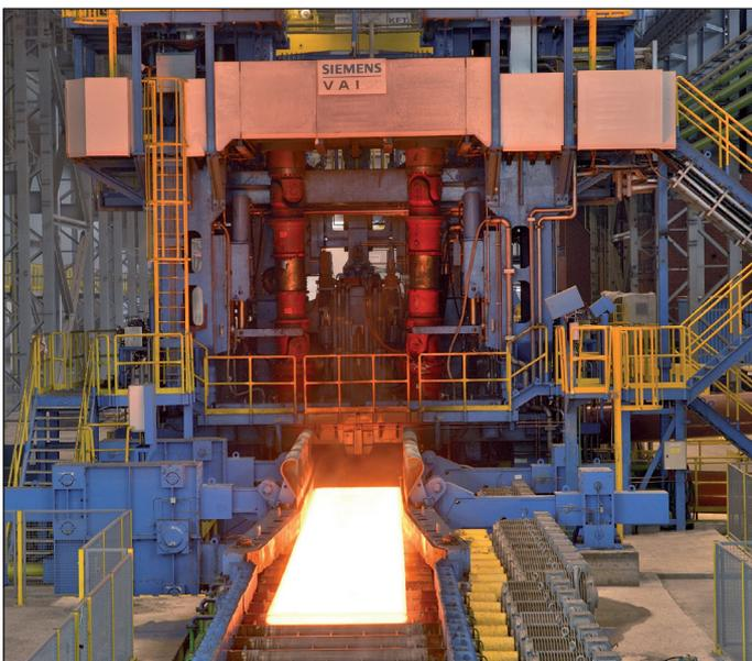
Siemens VAI will install a heavy edger on the reversing stand, as well as the hydraulic and lubricating systems.
