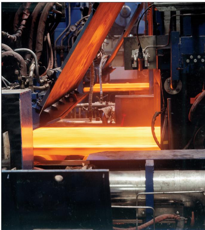
*ThyssenKrupp's casting-rolling mill in Duisburg-Bruckhausen: molten metal is turned into thin slabs of 48 to 53 mm thickness. Photo courtesy of ThyssenKrupp*
