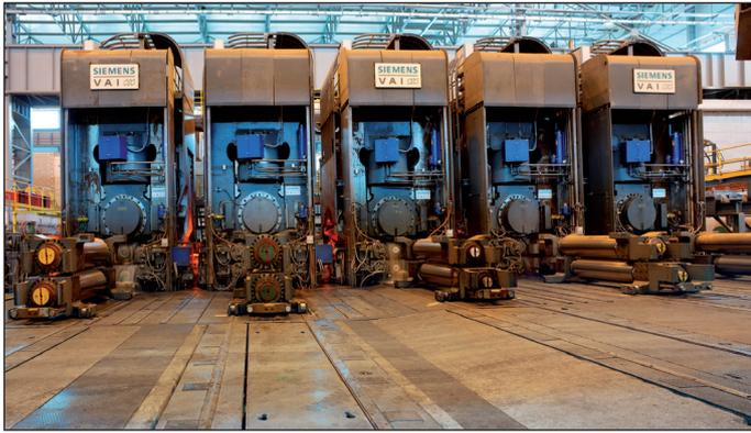
Siemens VAI-installed finishing stands in a hot-strip mill.
