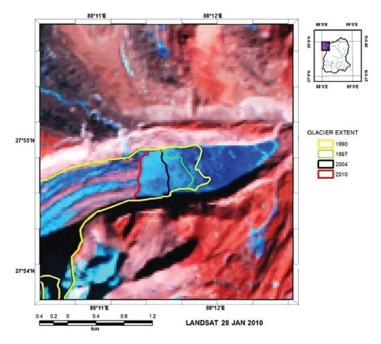
**Fig. 10.** The moraine-dammed lake at the terminus of South Lhonak Glacier (glacier No. 11 in Fig. 1) has expanded from  $0.50 \pm 0.05$  km<sup>2</sup> to  $1.08 \pm 0.07$  km<sup>2</sup> between 1990 and 2010. The expansion of the lake has reduced the glacier area by  $4.39 \pm 0.71$ %.
