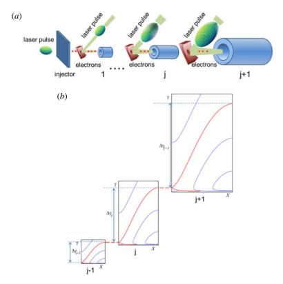
FIGURE 18. Multi-uneven stage accelerator comprising the injector and unequal stages. (a) Scematic of the multi-unequal stage LWFA accelerator. (b) Phase plots  $(X, \gamma)$  corresponding to the j - 1th, jth and j + 1th stages of the accelerator.
