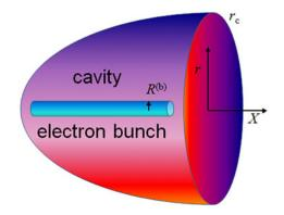
FIGURE 15. Electron bunch of radius  $R^{(b)}$  inside a cavity of radius  $r_c$ .
