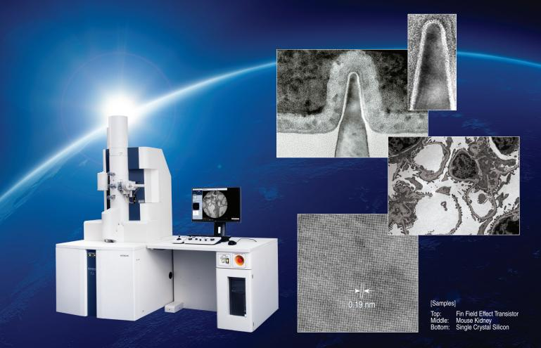
Hitachi's advanced electron optics and dual-mode lens technology redefine the boundaries of 120 kV TEM performance. With  $\leq$  0.19 nm on-axis resolution, the highest contrast in its class, and diverse analytical capabilities for Material Science and Life Science fields, the *HT7800* Series provides a complete solution for all your TEM imaging needs.
