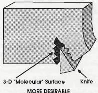
UNICRYL Resin provides sections suitable for either LM or TEM with proteins and nucleic acids exposed at the surface to give superior labelling and staining because the knife shears the resin slightly ahead of the knife edge to give much more of a three dimensional surface resulting in more surface area for the reaction to occur.
