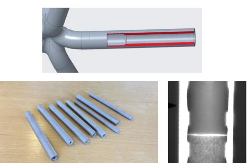
**Figure 9.** Detailed view of welding area (top). Printed AMDAs for welding and machining tests (bottom left) and X-ray of weld area (bottom right).
