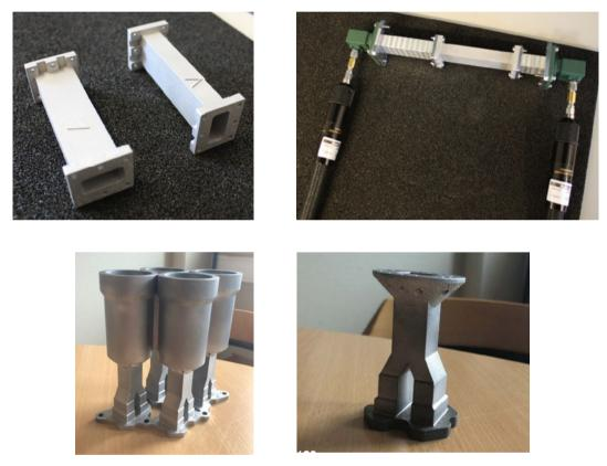
**Figure 8.** Printed waveguides (top left) and the test set-up (top right). New antenna array designed for AM (bottom left) and one printed AMDA for RF test (bottom right).
