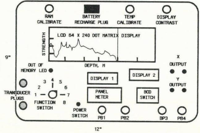
Fig. 3. Control unit lay-out for the DTR.
