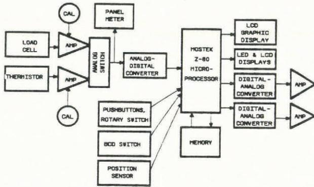
Fig. 2. Block diagram for the Digital Thermo-Resistograph.
