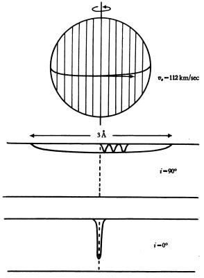
Fig. 1. Diagram illustrating the well-known Doppler broadening of spectrum lines due to axial rotation.
