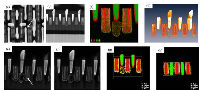
**Figure 2.** (a) Planar-TEM view of the sample; (b) Converted cross-section view of the planar sample in (a); (c) Cross-section EDS elemental map of the defect; (d) STEM tomography voltex visualization of the defect; (e), (f) Reconstructed OrthoSlice of the defect; (g),(h) EDS elemental tomography of the defect.
