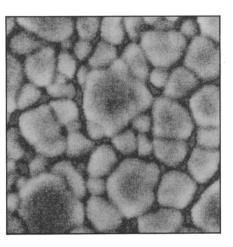
**ON THE COVER:** Scanning electron microscope image of Pb  $(Mg_{0.3}Nb_{0.6}Ti_{0.1}) O_3$ , relaxor ferro-electric ceramics used as electrostrictive actuators. For more information on this topic, see "Sensors, Actuators, and Smart Materials" by S. Trolier-McKinstry and R.E. Newnham, starting on page 27. Micrograph taken by Jie Chen and Martin Harmer of Lehigh University.
