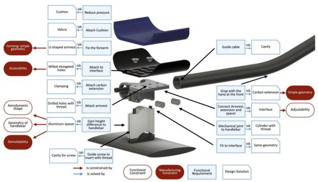
Figure 2. Function model and product architecture of a conventional aerobar
