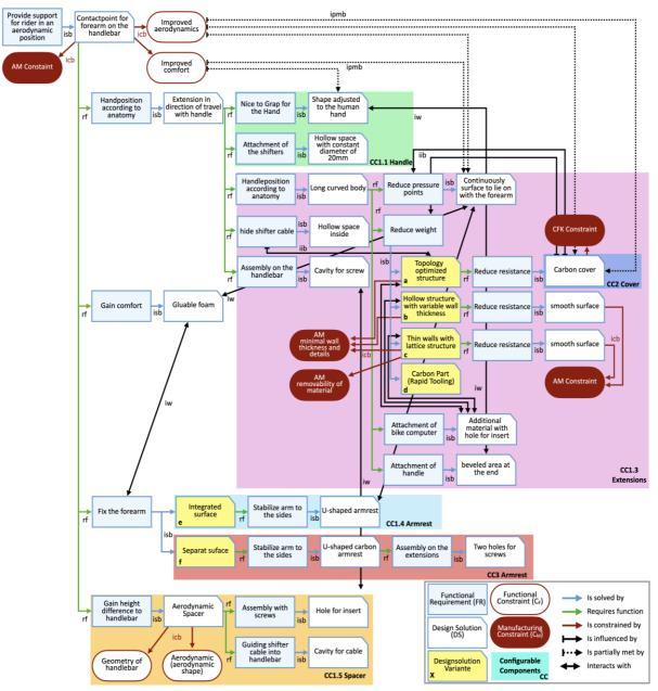
Figure 3. Redesigned EF-M for additive manufacturing
