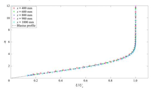
Figure 2. Mean velocity profiles of the laminar boundary layer over a flat plate at various streamwise locations, which are compared with the Blasius profile. Here,  $\eta = y(U_e/\nu x)^{1/2}$  is the non-dimensional distance from the wall.
