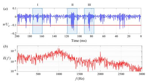
Figure 4. Time series (a) and power spectrum (b) of the hot-wire signal immediately above the disturbance source (x = 325 mm) at y = 0.5 mm.
