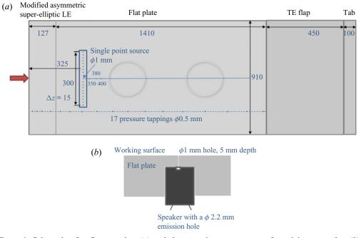
Figure 1. Schematic of a flat test plate (a) and the mounting arrangement of a miniature speaker (b). Dimensions are in millimetres. There are, in total, 19 orifices and miniature speakers across the span of the test plate, but only the centre speaker is used in this study. Two unused circular instrumentation plates are also shown.
