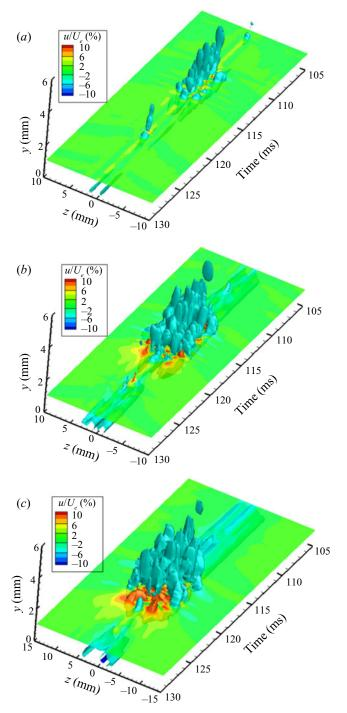
Figure 9. Three-dimensional structure of Spot II depicted by iso-surfaces of ensemble-averaged x-component velocity fluctuations at 10% (coral) and -5% (cyan) of the freestream velocity, where colour contour slices at y = 1 mm are superimposed: (a) x = 350 mm; (b) x = 380 mm; (c) x = 400 mm.
