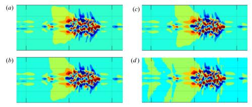
Figure 8. Effect of the number of ensemble average on the streamwise velocity contour of Spot II at x = 380 mm, y = 1.0 mm: (a) 20 ensembles, (b) 10 ensembles, (c) 5 ensembles and (d) no ensembles (a single realisation).
