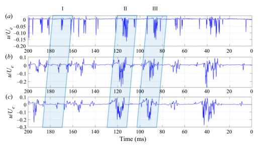
Figure 12. Streamwise velocity signals (a single realisation) in the boundary layer at y = 1.5 mm, showing the downstream development of Spot I, II and III: (a) x = 350 mm, (b) x = 380 mm, (c) x = 400 mm.
