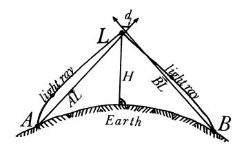
Fig. 1. A and B are the stations, H is the height of the signal L,  $\overrightarrow{AL}$  and  $\overrightarrow{BL}$  are uncorrected direction vectors and d is shortest segment between them.
