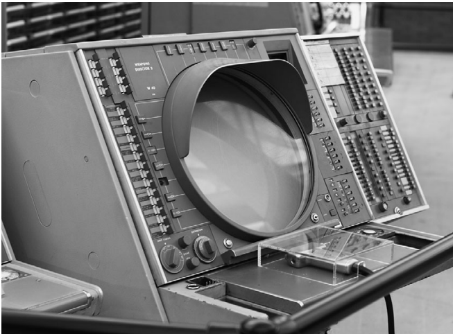
Figure 1.3 Situation display console of the AN/FSQ-7 computer, which was a part of SAGE. (Source: Computer History Museum, Photo by Joi Ito, 36 CC-BY 2.0)
