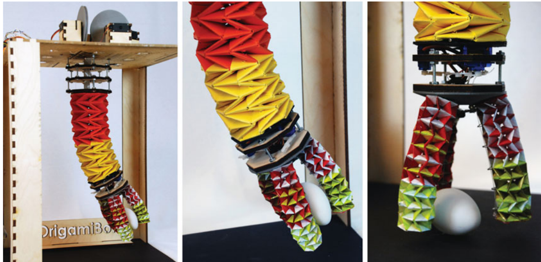
Fig. 1. OrigamiBot-II: Three-finger origami manipulator using the origami twisted tower for constructing the arm and fingers. Four servo motors, installed on the top of the frame, control the arm and three mini-servos control the three fingers for grasping an object.
