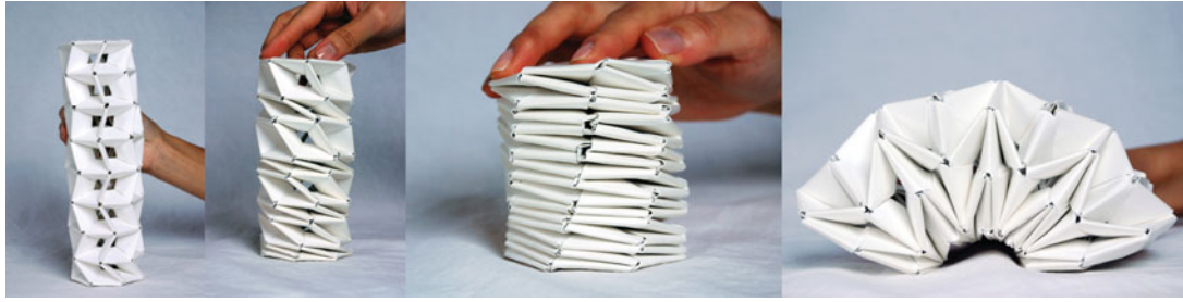
Fig. 2. Twisted tower in different configurations showing linear extension and contraction and bending. Each layer can be configured to be folded in one of the two directions.
