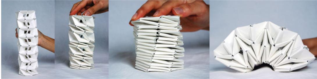
Fig. 2. Twisted tower in different configurations showing linear extension and contraction and bending. Each layer can be configured to be folded in one of the two directions.
