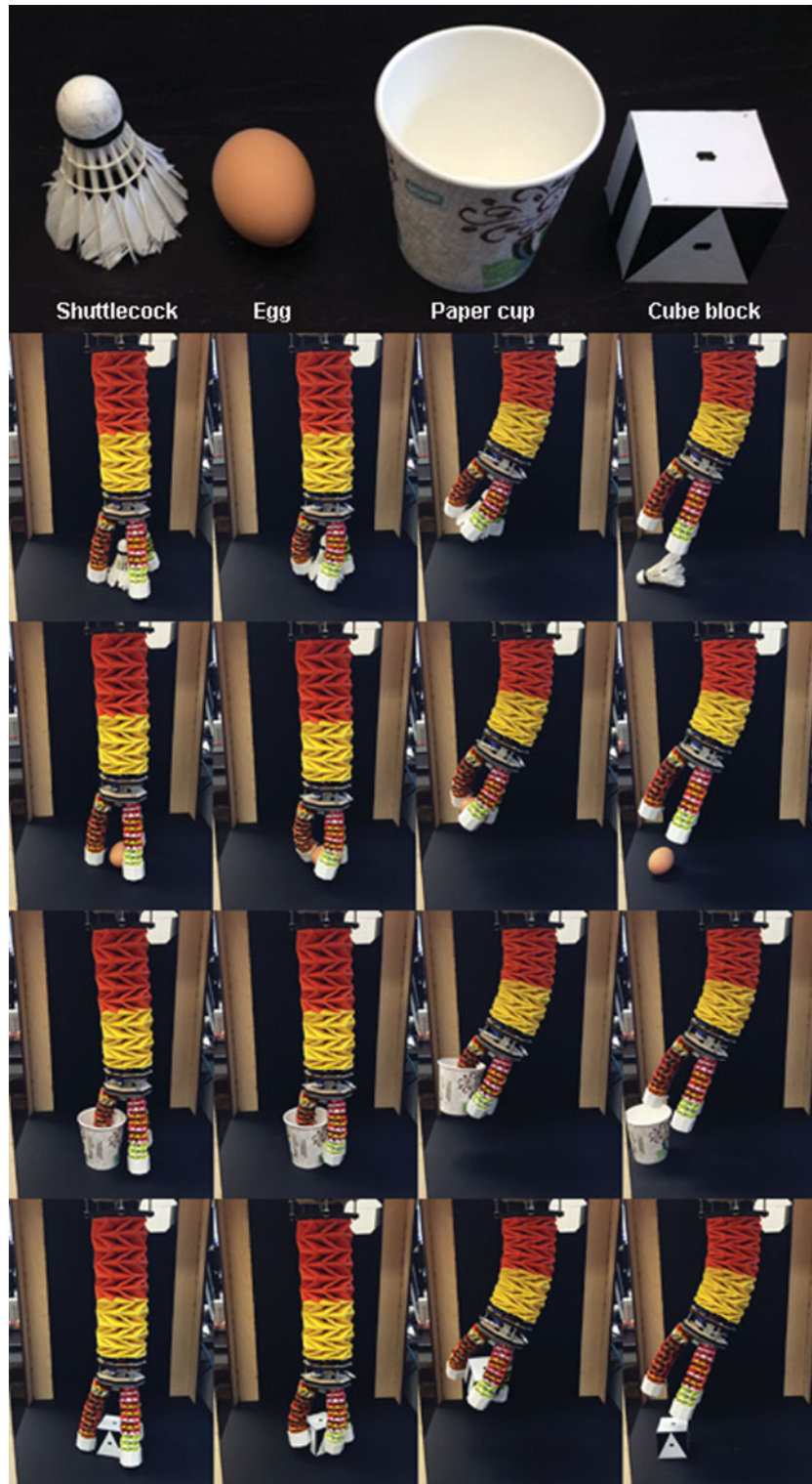
Fig. 9. Video-captured images showing physical demonstrations of the robot's manipulation capability for five different objects.
