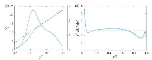
Figure 17. Box and grid sensitivity study for one-point statistics: (a) inner-scaled mean velocity profiles and streamwise velocity variances, and (b) log-law diagnostics function. The dashed line in (a) refers to the logarithmic fit  $U^+ = \log y^+/0.375 + 4.21$ . The dashed horizontal line in (b) denotes the inverse Kármán constant 1/0.375. The line style is as in table 2.
