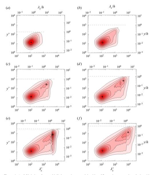
Figure 4. (*a*–*f*) Variation of pre-multiplied spanwise spectral densities of fluctuating streamwise velocity with wall distance, for cases A–F, respectively. Wall distances and wavelengths are reported both in inner units (bottom, left axes) and in outer units (top, right axes). The dashed line denotes the channel free surface. The crosses denote the positions of the inner and outer energetic sites. Contour levels from 0.2 to 2.0 are shown, in intervals of 0.2.
