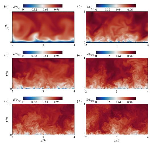
Figure 2. (a-f) Instantaneous streamwise velocity field (normalized by the mean free-surface velocity  $U_{FS}$ ) in a cross-stream plane, for the flow cases A–F, respectively, listed in table 1. Here, y = 0 corresponds to the no-slip wall, and y/h = 1 corresponds to the free surface. Note that only a limited part of the domain span is shown.
