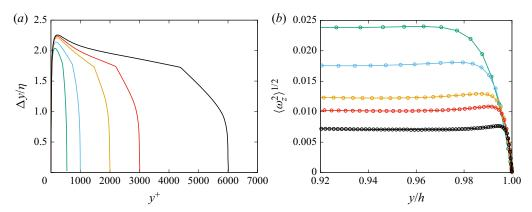
Figure 15. (a) Wall-normal grid resolution, in terms of grid spacing in local Kolmogorov units. (b) Detail of the root-mean-square spanwise vorticity near the free surface. The colour codes are as in table 1.
