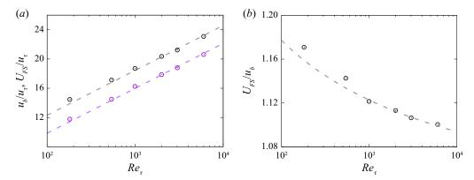
Figure 10. (a) Mean free surface velocity ( $U_{FS}$ ) and bulk velocity, and (b) their ratio, as functions of the friction Reynolds number. DNS data are shown as circle symbols, and the corresponding logarithmic fits are shown as dashed lines. Black is used for  $U_{FS}$ , and purple for  $u_b$ .
