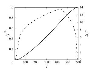
Figure 14. Distribution of wall-normal coordinate  $(y_j, \text{ solid line})$  and corresponding grid spacing  $(\Delta y, \text{ dashed line})$  for flow case F, as a function of the grid index (j).
