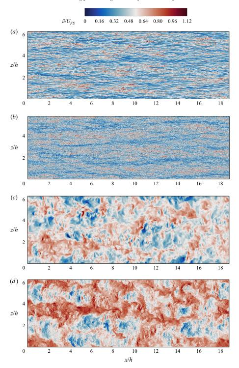
Figure 3. Instantaneous streamwise velocity fields in wall-parallel planes: (a,b) near the no-slip wall  $(y^+ = 15)$ , and (c,d) at the free surface (y/h = 1), for (a,c) flow case C  $(Re_{\tau} = 1000)$ , and (b,d) flow case F  $(Re_{\tau} = 6000)$ .
