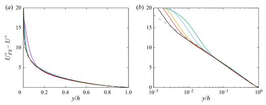
Figure 9. Defect velocity profiles for DNS of open channel flow, in (a) linear and (b) semi-logarithmic scale. The dashed grey line marks the outer-layer logarithmic fit  $U_{FS}^+ - U^+ = -0.128 - 1/0.375 \log(y/h)$ .
