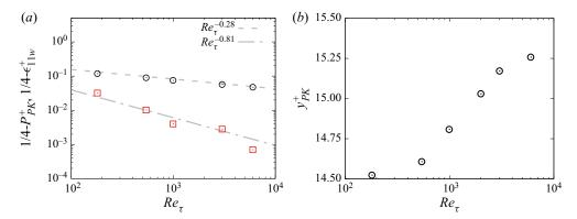
Figure 12. (a) Distributions of peak turbulence production ( $P_{PK}$ , squares), and wall dissipation of streamwise velocity variance ( $\epsilon_{11w}$ , circles). (b) Peak position of streamwise velocity variance. In (a), the dot-dashed and dotted lines denote fits of  $P_{PK}$  and  $\epsilon_{11w}$  in their tendency to the respective assumed asymptotic values.
