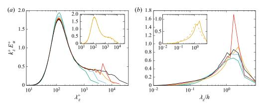
Figure 6. Pre-multiplied spectral densities of streamwise velocity at (a)  $y^+ = 15$  and (b) y/h = 0.28. The insets report a comparison with spectra in a closed channel at  $Re_{\tau} = 2000$  (solid lines indicate open channel, dashed lines indicate closed channel). The colour codes are as in table 1.
