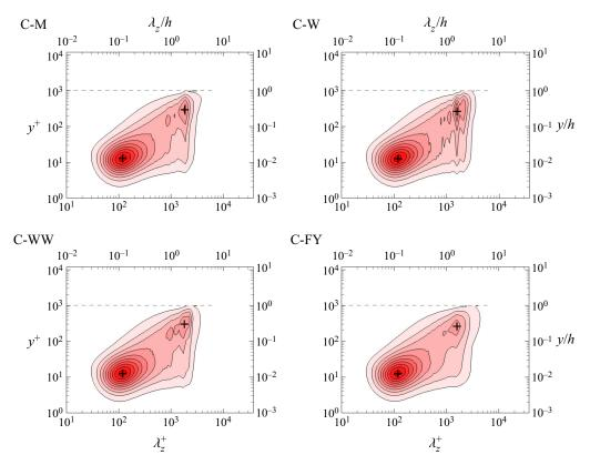
Figure 16. Variation of pre-multiplied spanwise spectral densities of instantaneous streamwise velocity with wall distance for the flow cases listed in table 2. Wall distances and wavelengths are reported both in inner units (bottom, left axes), and in outer units (top, right axes). The dashed line denotes the channel free surface. The crosses denote the positions of the inner and outer energetic sites. Contour levels from 0.2 to 2.0 are shown, in intervals of 0.2.
