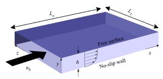
Figure 1. Definition of the computational set-up for DNS of open channel flow. Here, x, y, z are the streamwise, wall-normal and spanwise directions, respectively,  $L_x$  and  $L_z$  are the box sizes along the streamwise and spanwise directions, h is the channel depth, and  $u_b$  is the bulk velocity.
