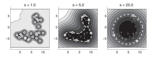
**Figure 3** Data description trained on a banana-shaped data set. The kernel is a Gaussian kernel with different width sizes s. Support vectors are indicated by the solid circles; the dashed line is the description boundary. *Source*: Tax (2001).
