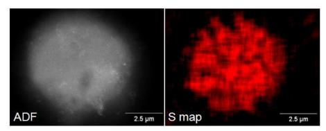
Figure.2 Z-contrast STEM image of red blood cell and x-ray mappings of S.
