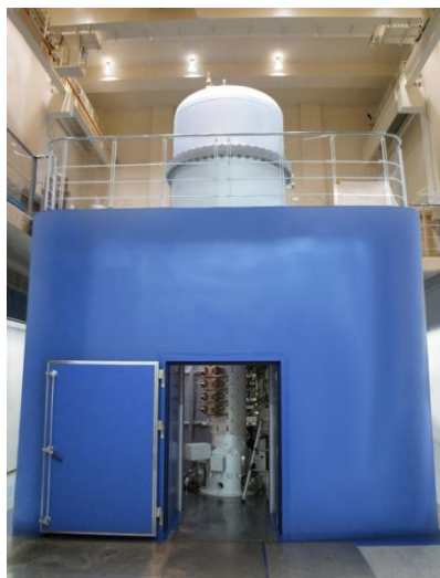
Figure 3. 1.2-MV field-emission holography electron microscope
