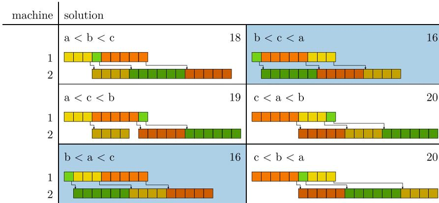
Fig. 6. Flow shop solutions for all possible permutations with the total execution length in the top right corner and optimal solutions with a blue background.
