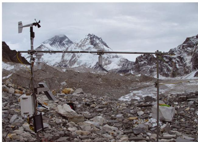
**Fig. 3.** Picture of the automated weather station on the debris-covered part of Changri Nup Glacier (5360 m a.s.l.) on 31 October 2010. The Everest summit is visible in the background.
