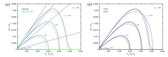
FIGURE 9. Growth rate of the parallel firehose instability for  $\beta_{\parallel} = 100$ . Kinetic solutions are solid blue lines. The temperature anisotropy is varied as  $a_p = 0.95$ ; 0.96; 0.97; 0.979 (the hard firehose threshold is at  $a_p = 0.98$ ). Four different fluid models are plotted, and all fluid solutions have dashed lines. (a) Hall-CGL (blue), Hall-CGL-FLR1 (green). (b) Hall-CGL-FLR2 (blue), Hall-CGL-FLR3 (black).
