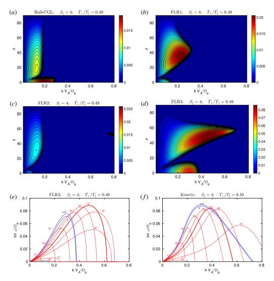
FIGURE 10. The growth rate plotted in the  $k-\theta$  plane, with fixed  $\beta_{\parallel}=4$  and  $a_p=0.49$  (the hard firehose threshold is at  $a_p=0.5$ ), showing the parallel and oblique firehose instability. Four different fluid models are plotted. (a) Hall-CGL; (b) Hall-CGL-FLR1; (c) Hall-CGL-FLR2, (d) Hall-CGL-FLR3. We do not provide a contour plot for kinetic theory. Nevertheless, the bottom figures show solutions for several propagation angles. (e) Hall-CGL-FLR3 model, (f) kinetic.
