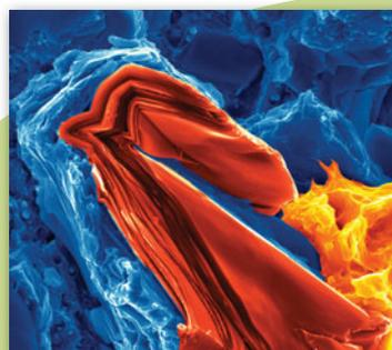
This image shows a fractured surface of a magnesium matrix composite reinforced with titanium aluminum carbide,  $Ti_2AlC$ , a layered ternary carbide MAX phase. The dragon is a kinked  $Ti_2AlC$ , and the surrounding material, including the fire, is the Mg matrix. Credit: Babak Anasori and Michel W. Barsoum.
