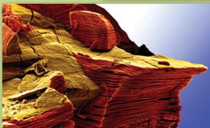
When the layered ternary compound,  $Ti_3AlC_2$ , is placed in hydrofluoric acid, the Al layers are selectively etched away, resulting in 2D layers of  $Ti_3C_2$  weakly bonded to each other. The image shows a number of these particles, where exfoliation is obvious. Credit: Babak Anasori, Michael Naguib, Yury Gogotsi, and Michel W. Barsoum.
