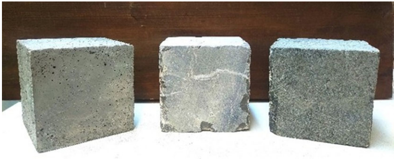
Figure 5. The cube samples from right to left: granite, marble, and concrete.
