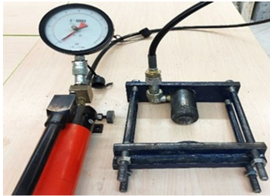
Figure 3. Hydraulic jack and metal frame for confining pressure applications.
