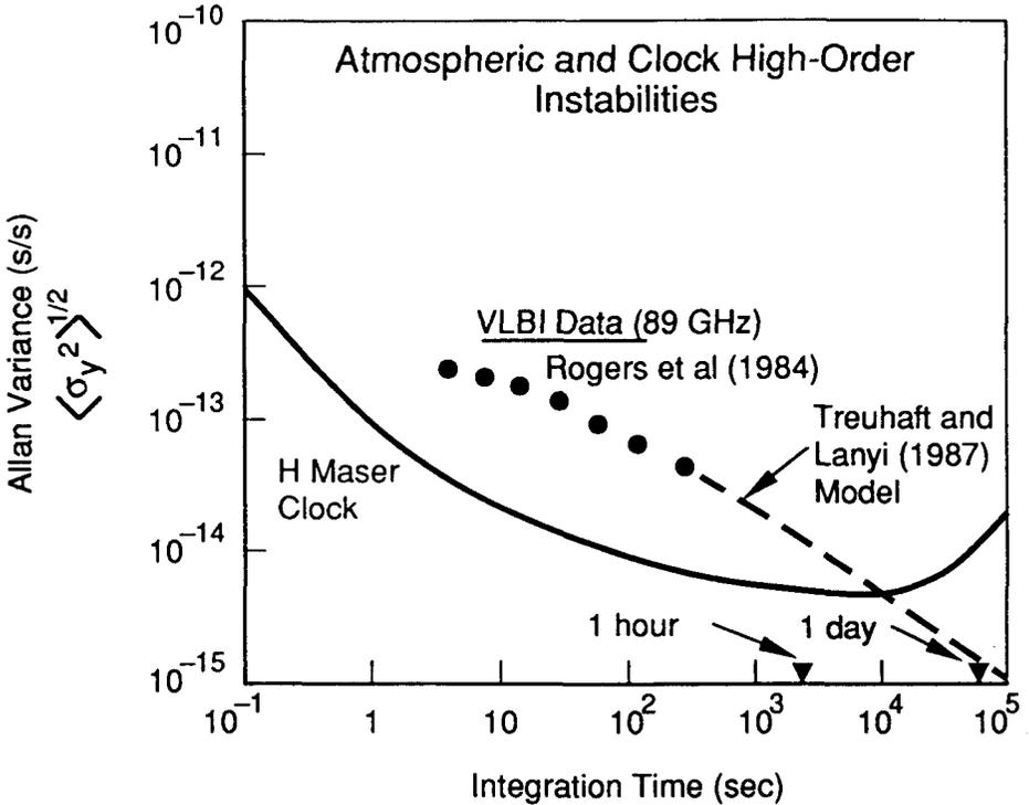
Fig. 1 : Allan Variance functions showing the fractional frequency instabilities of a VLBI station clock and of the wet component of the troposphere
