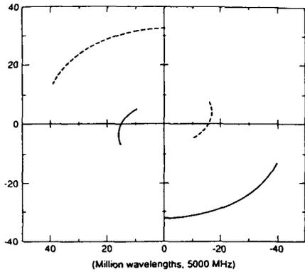
FIG. 4.  $u - v$  coverage corresponding to the phase-referenced dirty map of Algol.
