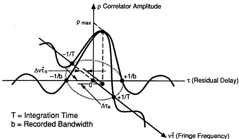
Fig. 2 : Concept of the delay and delay-rate tracking to find weak VLBI fringes with the strong reference source residuals ( $\Delta \tau_R, \Delta \nu \tau_R$ ).
