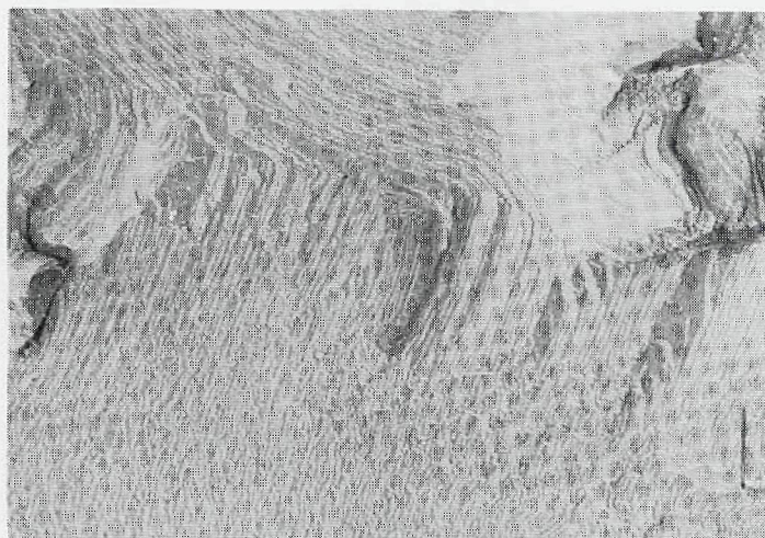
Figure 2: TEM micrograph of the reversed hexagonal LC of fenoprofen calcium at 250°C. Bar represents 200 nm.
