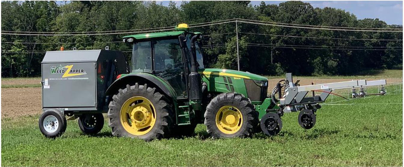
**Figure 2.** The model 6R30 Weed Zapper™ used in this experiment. The generator is attached to the back of a John Deere® 5100R tractor with a three-point hitch. The 4.6-m electric copper boom is attached to the front of the tractor with a three-point hitch. The Weed Zapper™ was purchased from Old School Manufacturing (Sedalia, MO, USA).
