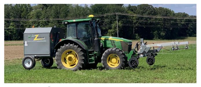
Figure 2. The model 6R30 Weed Zapper<sup>™</sup> used in this experiment. The generator is attached to the back of a John Deere® 5100R tractor with a three-point hitch. The 4.6-m electric copper boom is attached to the front of the tractor with a three-point hitch. The Weed Zapper<sup>™</sup> was purchased from Old School Manufacturing (Sedalia, MO, USA).
