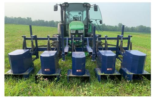
Figure 1. The interrow mower used in this experiment, attached to a John Deere® 5100R tractor with a three-point hitch. The mower is powered with a hydraulic system and was custom made by IRM X4, R-Tech Industries (Homewood, MB, Canada).
