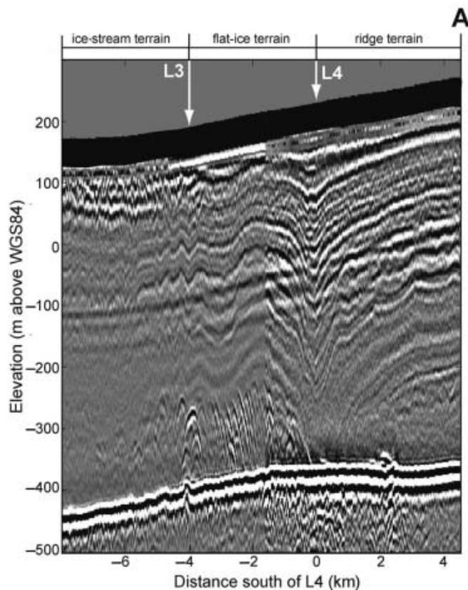
**Fig. 4.** 2 MHz radar profile along a section of line A (as shown in the box outlined in Fig. 3a) crossing L4 and the northernmost KIS margin (L3). The prominent return at approximately  $-100$  m elevation is a glitch in the transmitter. Data in the upper  $\sim 80$  m (covered by a black band) are not resolved by the radar system.
