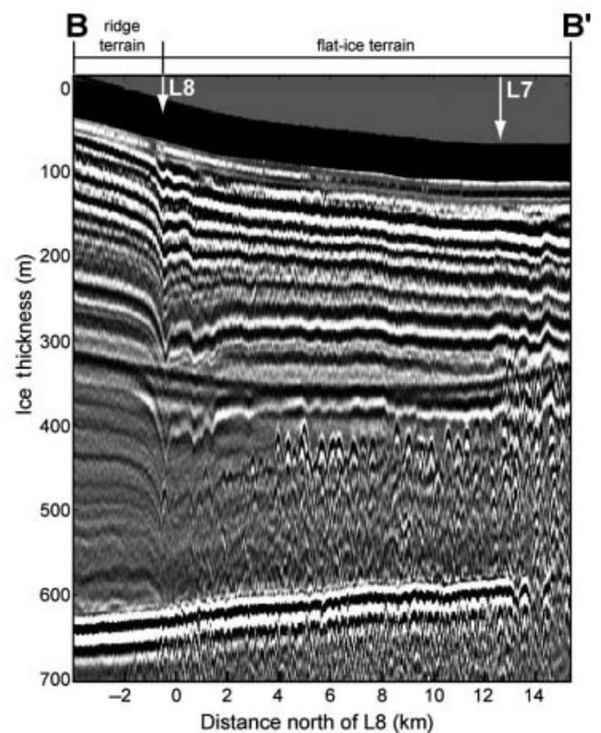
**Fig. 5.** 2 MHz data along line B in the Goosefoot crossing L7 and L8 (Fig. 1a). Note the prominent return at  $\sim 300$  m depth is a glitch in the transmitter. Data in the upper  $\sim 80$  m (covered by a black band) are not resolved by the radar system.
