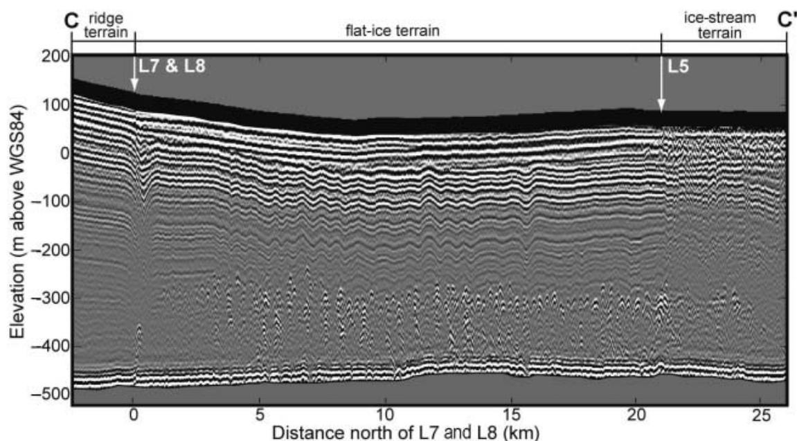
**Fig. 6.** 5 MHz radar profile along line C in the Goosefoot crossing L5, L7 and L8. Data in the upper ~80 m (covered by a black band) are not resolved by the radar system.
